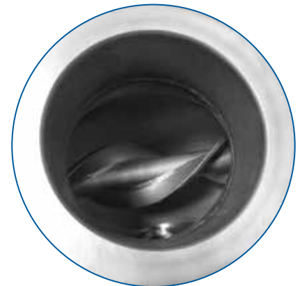
Inside view of non-ragging impeller
