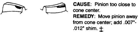
+Use the smaller tolerances for gear diameters in the 6"-8" range. Use the larger tolerances for gear diameters over 20". If correct tooth contact pattern cannot be achieved, consult factory.
