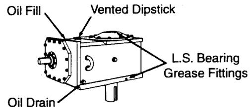
**NOTE: Oil Fill and Dipstick Positions Reversed on Sizes MB-58 and MB-59**
