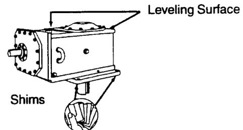
Figure 4 Shimming units
