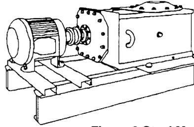
Figure 3 Steel Mounting
