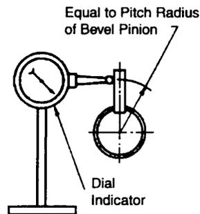
2. Rotate the bevel pinion shaft back and forth while holding the bevel gear shaft immobile. Read the backlash (tooth clearance) on indicator. Required backlash is etched on outer diameter of the bevel gear. Measure at three locations, 120° apart on the gear and use the minimum measured value for reference at adjustment.
