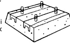
**Motors and other components mounted on motor plates may become misaligned during shipment. ALWAYS check alignment after installation. Refer to section (3) for coupling alignment instructions.**
